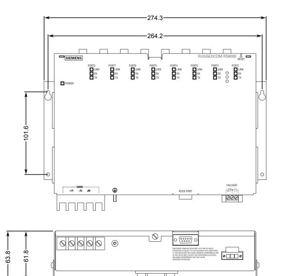
Figure 5.3 Panel and Din Rail Mount Dimensions
